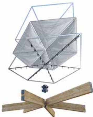
In detail – exploded roof section
