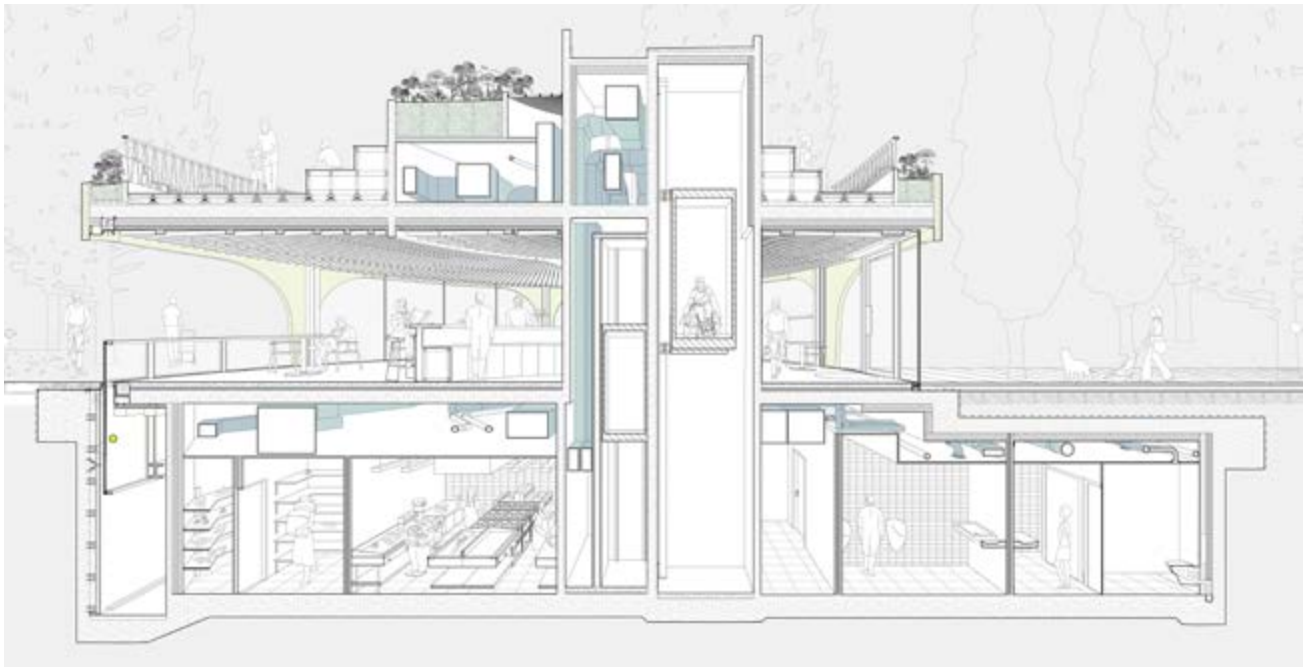
Cutaway showing the roof garden, restaurant with its sliding glazed walls, and kitchens below ground
