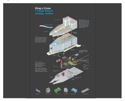
The focus for energy efficiency and sustainability at King's Cross is an on-site Energy Centre. The centre houses a Combined Heat and Power (CHP) plant. In time, the CHP plant will provide 100 per cent of the development's heat and hot water needs and 80 per cent of its electricity. Each building at King's Cross will be connected to the Energy Centre through a hot water distribution network.
