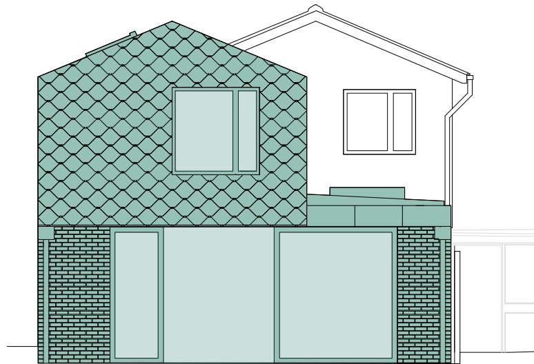
Rear elevation — the two-storey house volume was replicated and offset from the existing house
