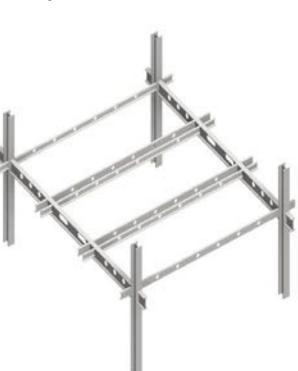
Figure 8.5 Supporting steelwork
